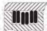
YHKD Series QHKD Series Internal - Heavy Duty 1 set = 3 individual rings (2 rings rotate with bore & 1 ring rotates with shaft)
