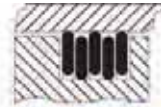
YHK Series QHK Series Internal - Medium Duty 1 set = 5 individual rings (3 rings rotate with bore & 2 rings rotate with shaft)
